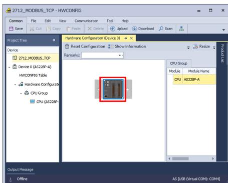
Figura 116 – Tela *HWCONFIG* (*Modbus TCP*)
