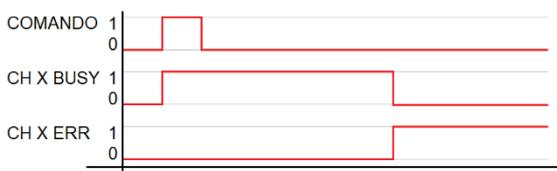
Figura 152 – Comportamento dos bits “CH X BUSY” e “CH X ERR”
